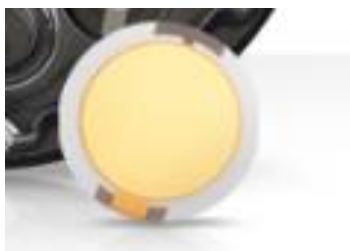
Figure 2.3: Quartz crystal microbalance (QCM) gold device 60 .
