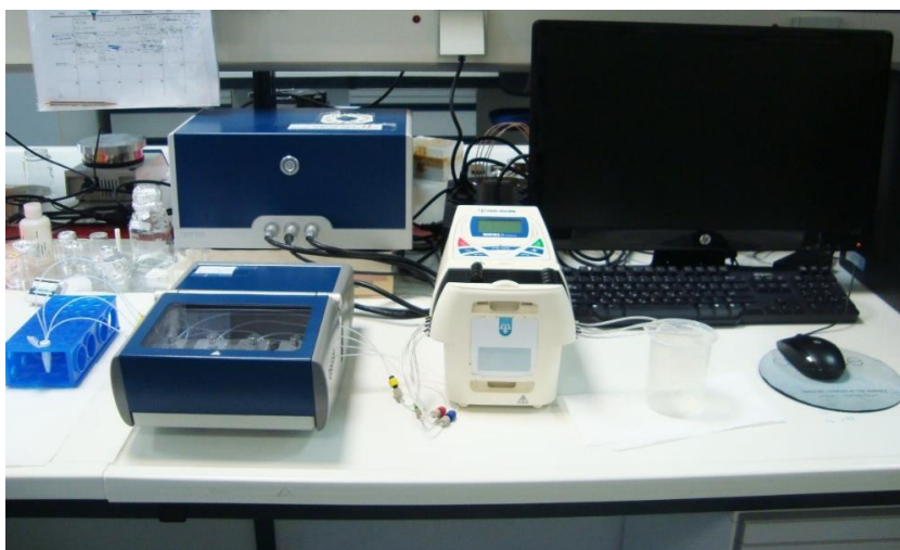
Figure 2.4: Experimental equipment for acoustic experiments. Q-Sense E4 instrument and peristaltic pump.
