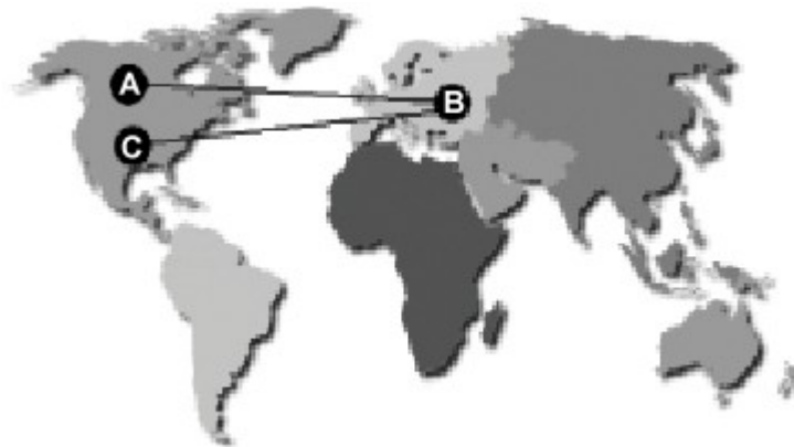
Figure 5.1: Illustration of inefficient routing in today's unstructured P2P systems
