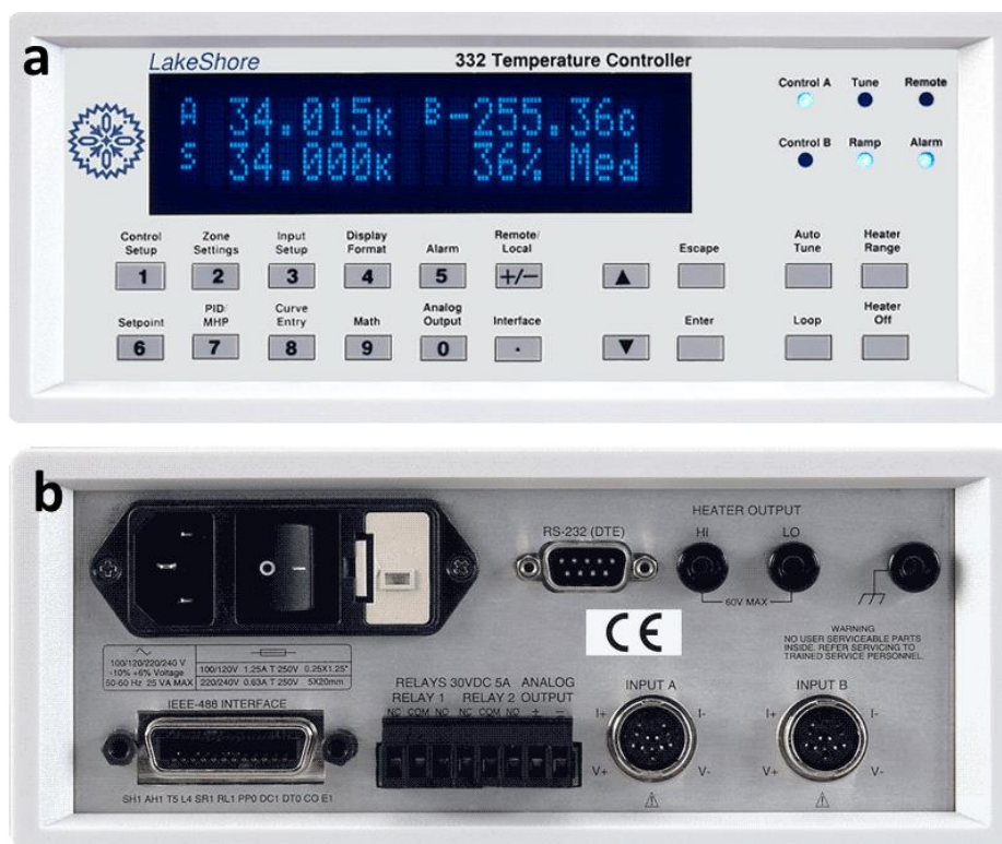
Figure B.1 a) Front panel of Lakeshore 332 Temperature Controller. The first column of numbers displayed refers to the actual temperature (A) whereas below this indication is the temperature set point (S) in units of Kelvin (K). The second column refers to the temperature of the sample and the total percentage of the output electrical power that was provided by the controller. The user may choose which panel will be displayed: the one which refers to the cryostat's temperature (Loop A) or the one which corresponds to the sample's temperature (Loop B).
