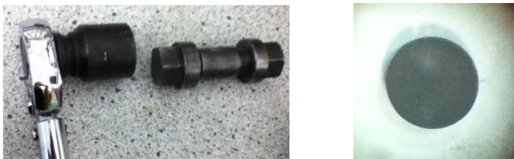
Figure 2.11 Left: The 5mm home made steel press. Also shown part of the torque key that was used to apply specific values of pressure. Right: A 5 mm diameter pellet of \beta - \text{NaMnO}_2 pelletized with the press as seen from the stereoscope.
