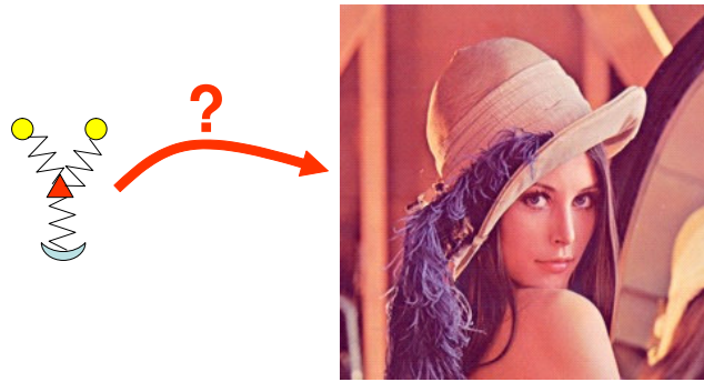
Fig. 1.8: We can model a face as a graph consisting of 4 objects: nose, mouth and two eyes. Each object is assumed to have a specific appearance, while some of the objects are connected to each other with springs. These springs try to keep the objects at an ideal relative distance. For detecting faces, we then need to locate that graph inside the image, but without stressing the springs too much.
