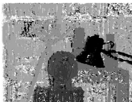
Fig. 1.7: If we try to estimate disparity based only the data terms of the energy function, then a noisy disparity map will almost surely be produced. Here we show the resulting disparity for the left and right image of figure 1.1. To ensure a better result, we must also take contextual constraints into account.
