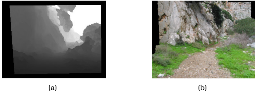
Fig. 5.5: (a) Depth map Z_0 of a local model (black pixels do not belong to its valid region dom_0 ). (b) A rendered view of the local model using an underlying triangle mesh
