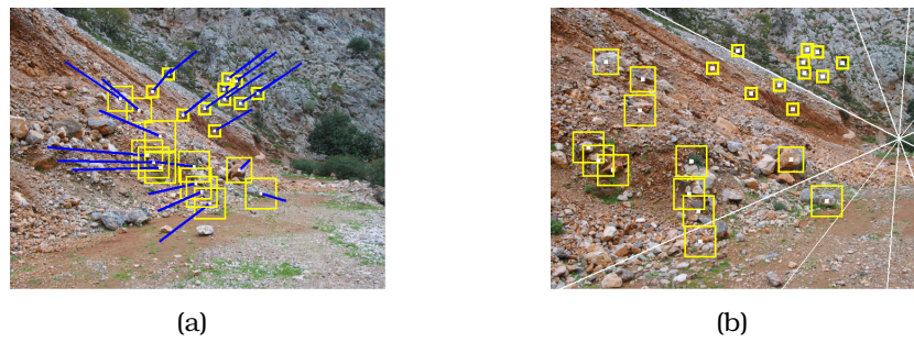
Fig. 5.7: (a) Image I_k along with computed optical flow vectors (blue segments) for all points marked white. (b) Image I_{k+1} along with matching points (also marked white) for all marked points of (a). A few epipolar lines are also shown. In both images, the yellow square around a point is analogous to the point's estimated scale factor (10 scales S = \{1, 0.9^{-1}, \dots, 0.1^{-1}\} have been used).
