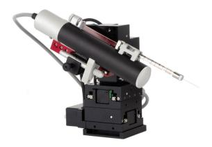
Figure 3.9: Micromanipulator siringe pump, image by AnimaLab.
