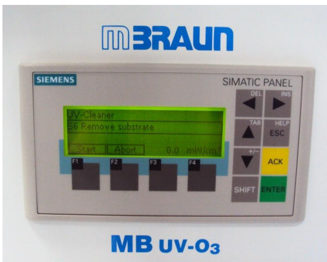
Figure 5.10 Settings screen of MBRAUN UV-O 3 cleaner
