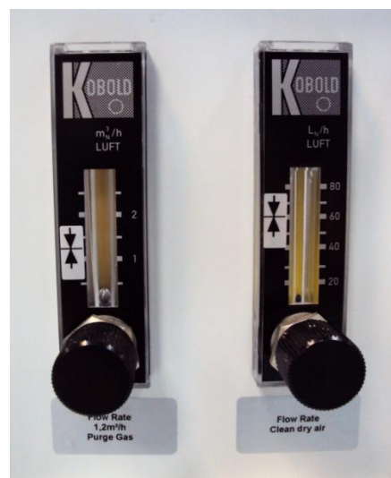
Figure 5.11 Air flow settings of MBRAUN UV-O 3 Cleaner.
