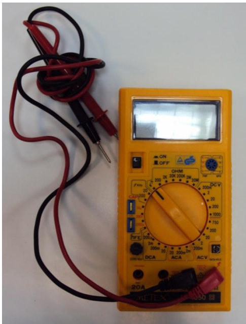
Figure 5.4 Multimeter used to ensure that the ITO-glass substrates are facing upwards.
