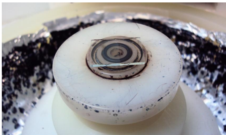
Figure 5.17 Proper positioning of the glass substrate on the rotation mechanism.
