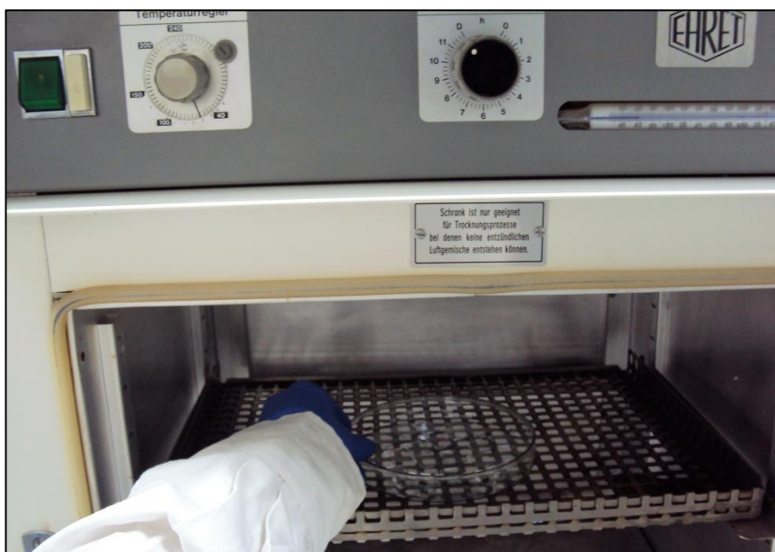
Figure 5.8 Placement of devices in the oven (120°C for 15 minutes) after cleaning.
