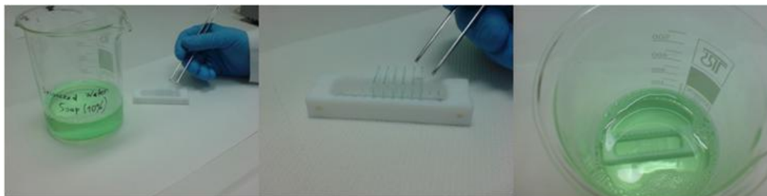
Figure 5.6 Insertion of the substrates into the holder and submersion in soap water.
