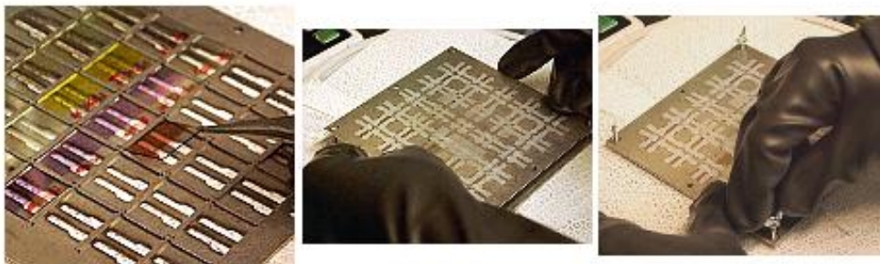
Figure 5.28 Shadow mask in which the substrates are placed in order to undergo metal deposition via VTE method.
