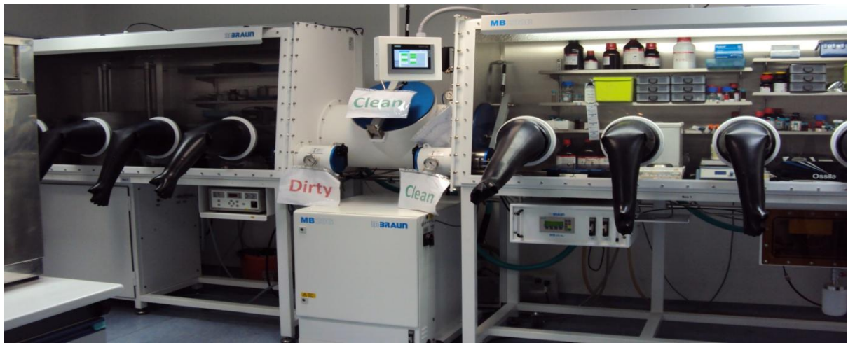
Figure 5.1 The glove boxes utilised throughout the experimental procedure. Glove Box No1 (right) contains the UV-O3 cleaner and the spin coater used for the deposition of the active layer. Glove Box No2 (left) contains the Vacuum Thermal Evaporator used for the deposition of the Ca Interlayer and Ag cathode.
