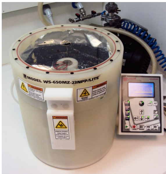
Figure 5.15 Spin coater used for the deposition of the HTL.
