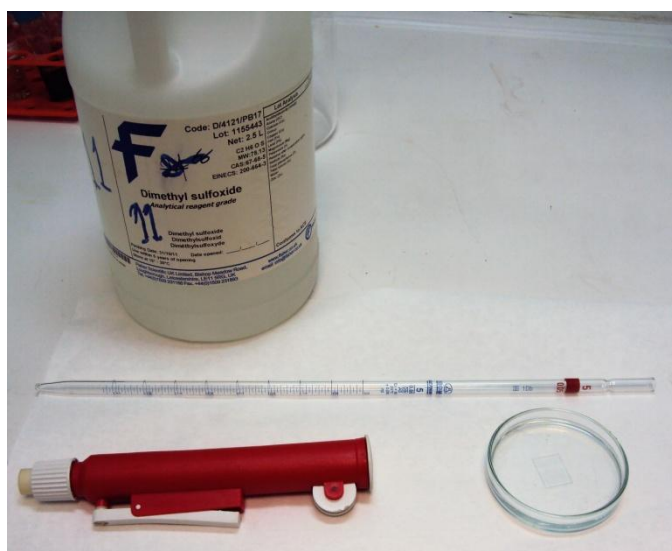
Figure 5.20 Equipment used for treatment of substrates with DMSO.
