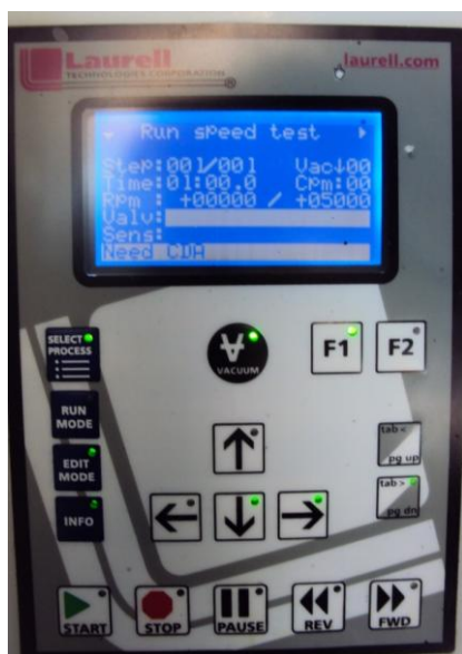
Figure 5.16 Settings screen of spin coater. Substrates were set to spin for 60 seconds at 5000rpm.
