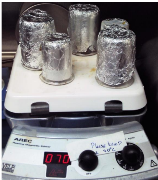
Figure 5.25 The PTB 7 -PC 60 BM blend is kept under dark conditions stirring on a hotplate at 70°C overnight.
