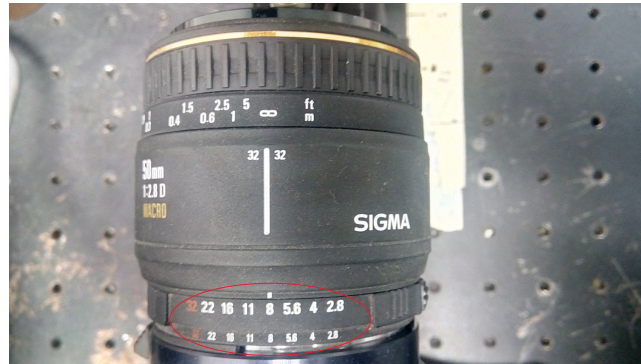
Figure 3.7: Diaphragm values in a camera
