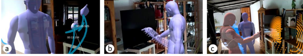
Figure 4: The AvatAR analysis environment. (a) Ghost Preview technique with two pinned hand ghosts touching the display. (b) Specter Visualizations technique of just the avatar's hands, showing past and future time frames as semi-transparent instances of the hands. (c) Gaze Visualization for two persons, one looking at the display and one looking at the other person.
