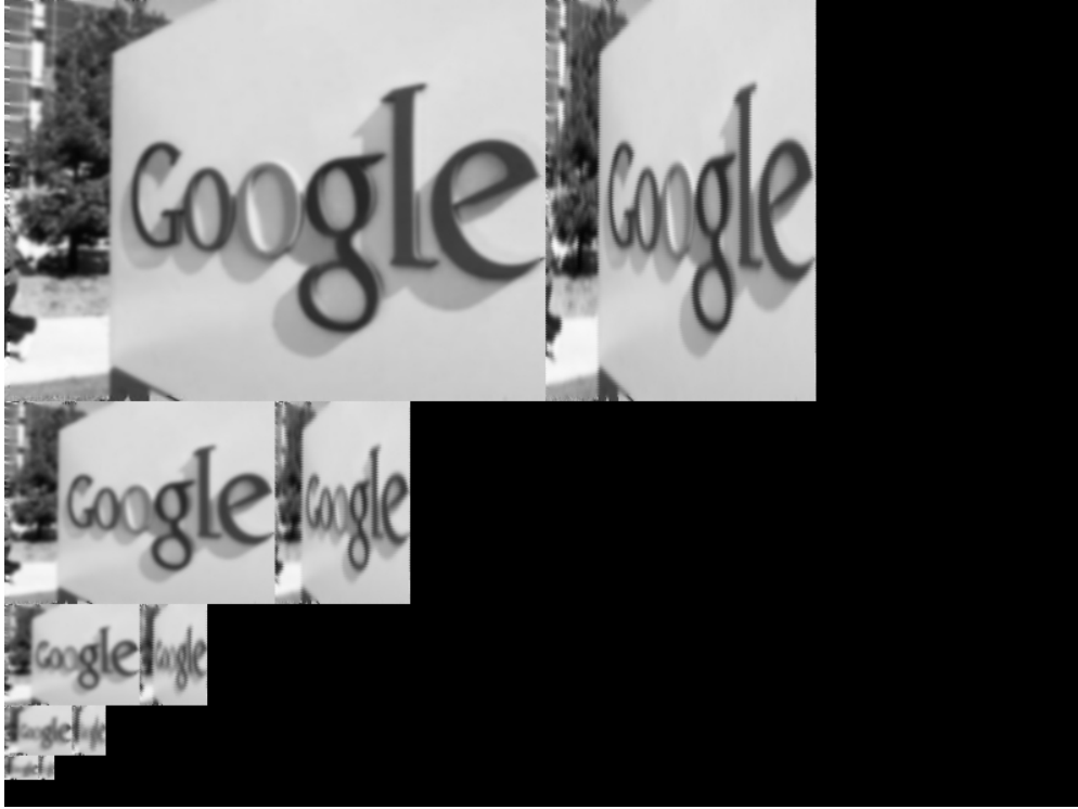
Figure 4.7: The result of Half-Octave Gaussian pyramid implementation on the L channel of the image [42]: the output is an image consisting of all the convolved images created at each k level of the pyramid.
