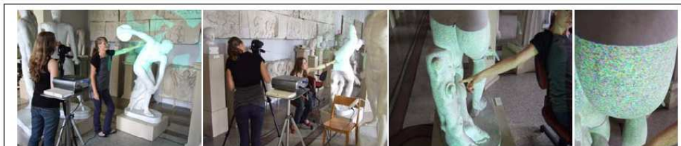
Fig. 2: The acquisition process. The string helps to keep the camera at the same distance from the chosen surface point. The Autofocus is switched off, both for greater speed and greater accuracy.
