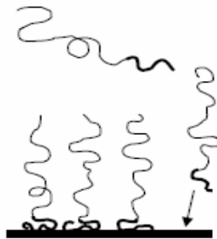
Figure 4. Preparation of polymer brushes by physisorption.
