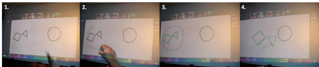
Figure 13: Selecting some elements in a sketch using the pen, and processing them using two fingers
