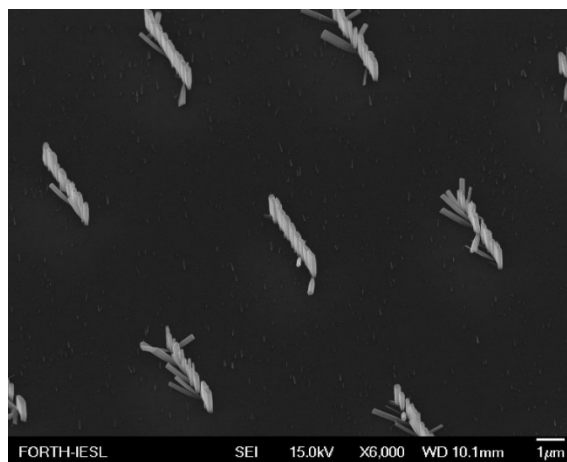
Figure 5.4: SEM image in tilted view of GaN fins grown on masked Si (111) substrates with 150\text{ nm} width, 3\mu\text{m} length and 6\mu\text{m} pitch.
