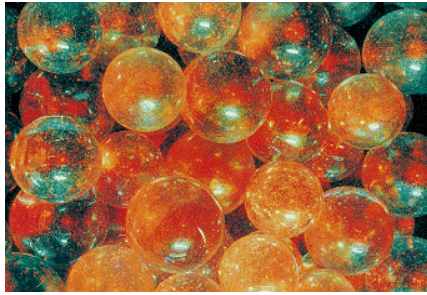
Fig. 3.2: Model picture of a random lasing medium. The microparticles both scatter and amplify light [2].
