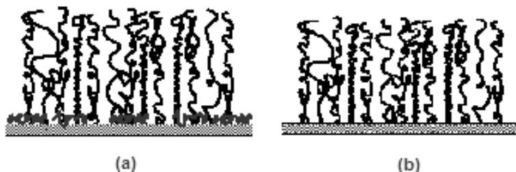
Figure 1.1: Polymer brush systems (a) adsorbed diblock copolymers and (b) end-grafted polymers.
