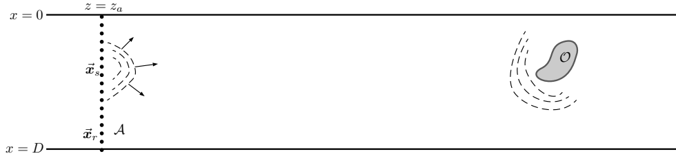
Figure 2.2: Active imaging setup in an infinite strip.
