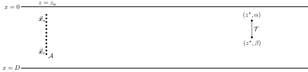
Figure A.2: Active imaging setup for a vertical screen, in an infinite strip.
