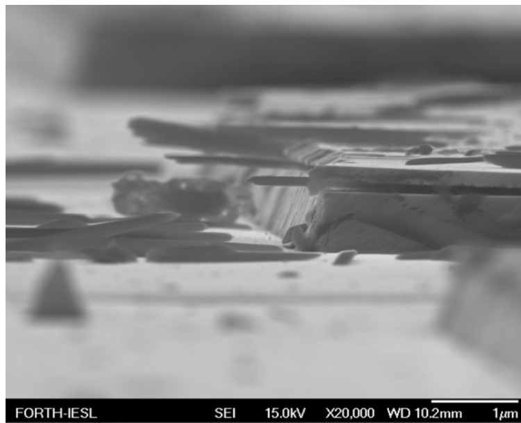
FIG.5.15. SEM image of extruded InGaN sacrificial layer sheets from the mesa facets.
