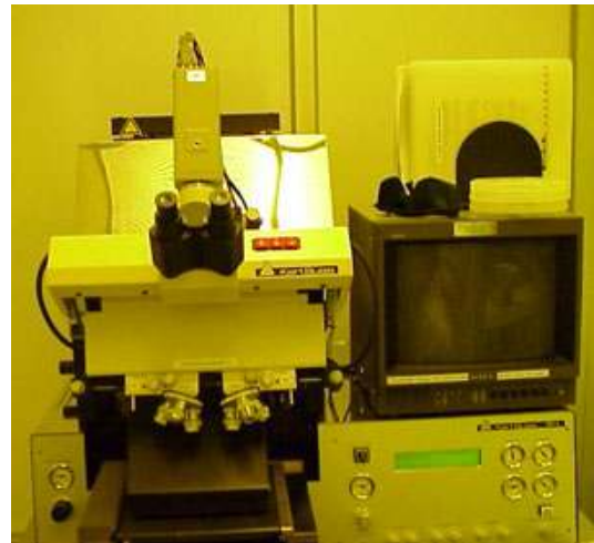
Fig. 2.4 The MA-6 mask-aligner of Karl Suss.
