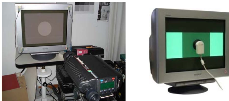
Figure 2.1 The technical equipment used for the experiments and the calibration of the monitor. PR650 (left), ColourCal (right) and the screen.
