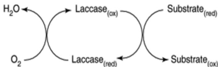
Figure 1: Schematic representation of laccase-catalyzed oxidation redox cycles for substrates oxidation.
