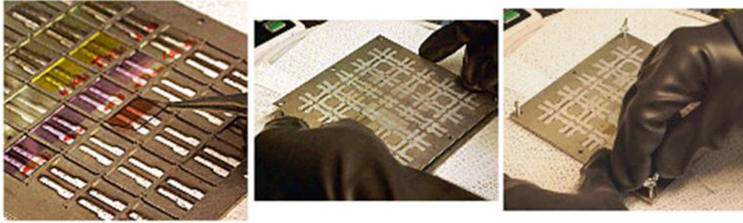
Figure 43: The placement of substrates in a cathode deposition mask
