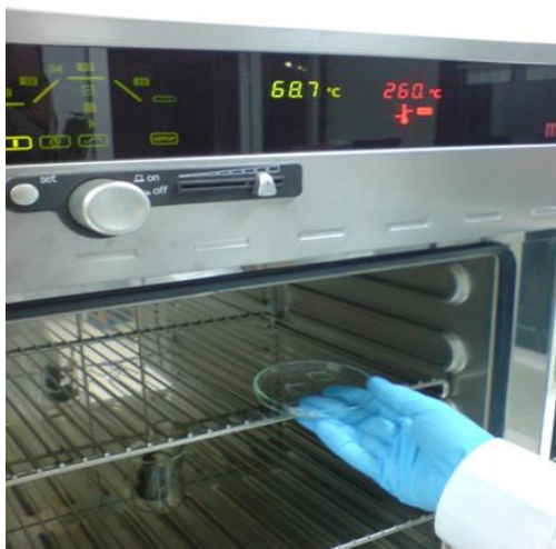
Figure 38: The substrates are placed to a holder for drying
