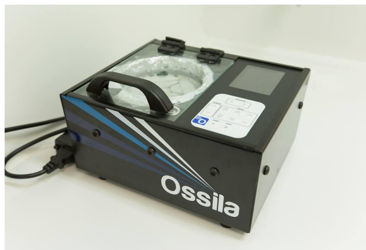
Figure 30: The spin coater by Ossila was used for deposition of perovskite materials
