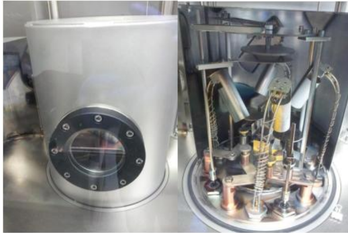
Figure 33: The MB-EcoVap evaporator under high vacuum (left) and with the vacuum chamber open(right).
