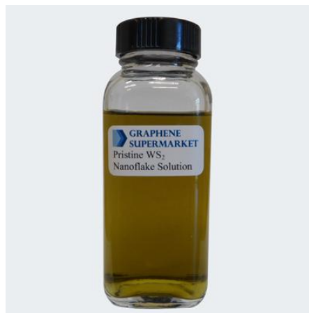
Figure 64: The solution of WS_2 flakes
