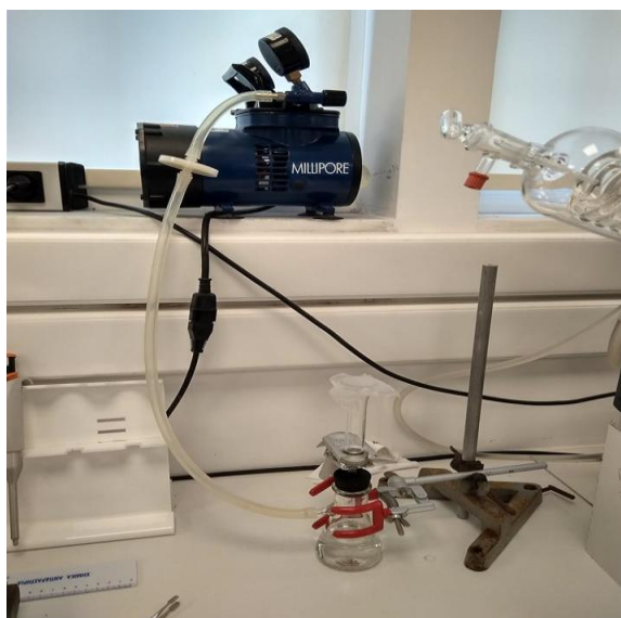
Figure 28: The vacuum filtration and the pump system that was used.
