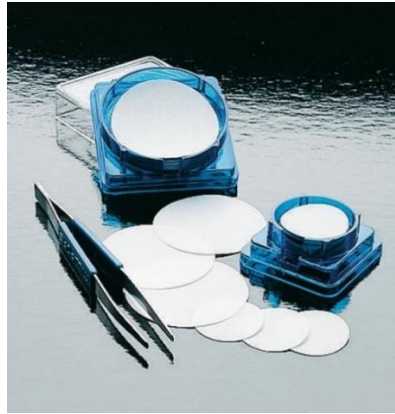
Figure 49: The mixed cellulose membranes that used for experimental procedure
