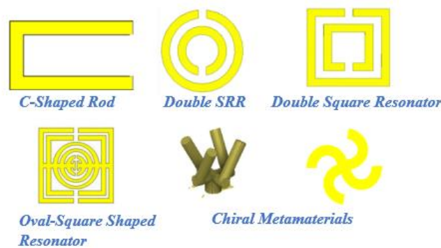
Figure 6.2.3: Example Of Different Metamaterial Geometries (meta-atoms) [47], [49], [51]
