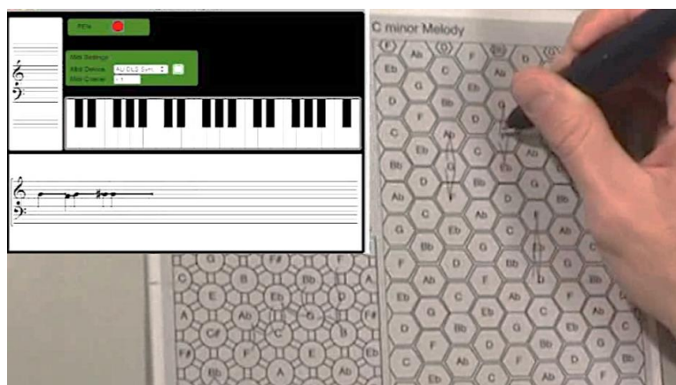
Figure 13. The PaperTonnetz system in practice. The user draws music paths using a digital pen and listens to the musical sequence on the computer.
