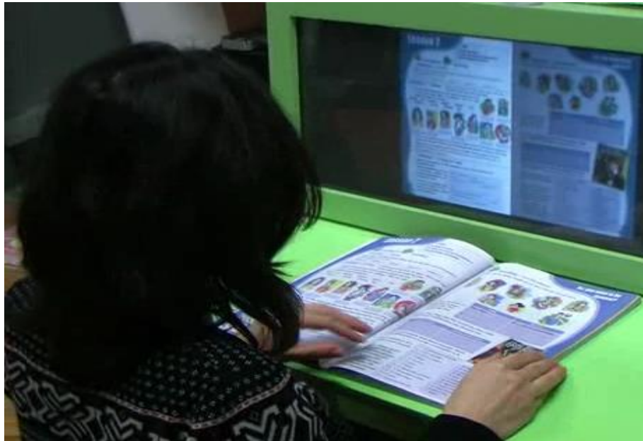
Figure 41. While the user changes the page of a book placed on the desk, SESIL recognizes the opened page and displays its digital image on a nearby screen.
