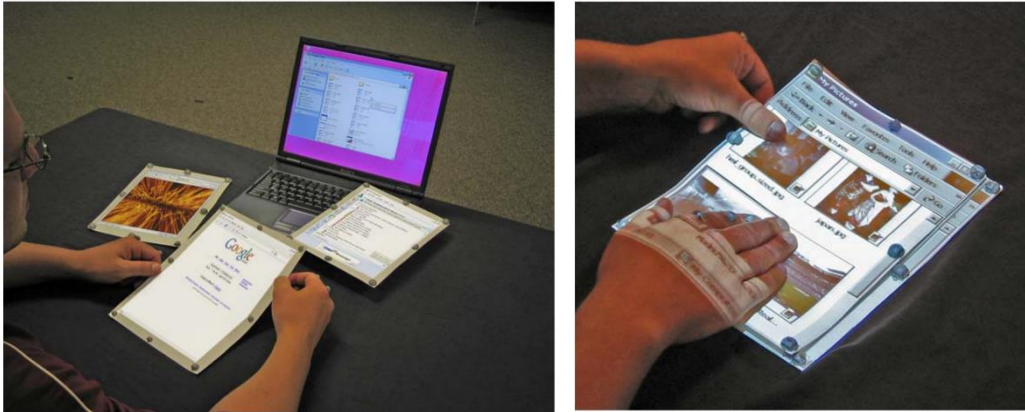
Figure 6. Left: PaperWindows prototype. Right: A paper window is placed on top of a blank page and its content is copied using a rubbing gesture.
