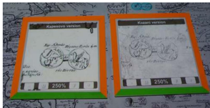
Figure 12. PaperView: supplements physical printed surfaces (e.g., maps) with digital information, through the use of pieces of plain paper that act as personal, location-aware, interactive screens.
