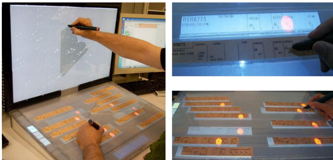
Figure 11. The Strip'TIC system providing computer aided support for air traffic controller through digitally augmented paper strips.
