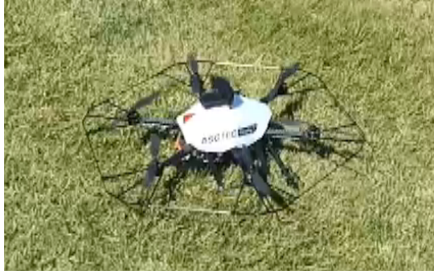
Figure 6.3.6: Outdoor experiments UAV with dual camera set-up; Firefly.
