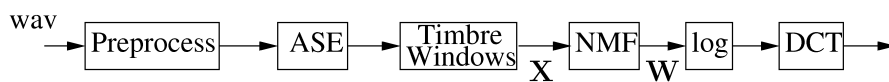
Figure 6.3: Calculation of the features used for the statistical model of musical genres
