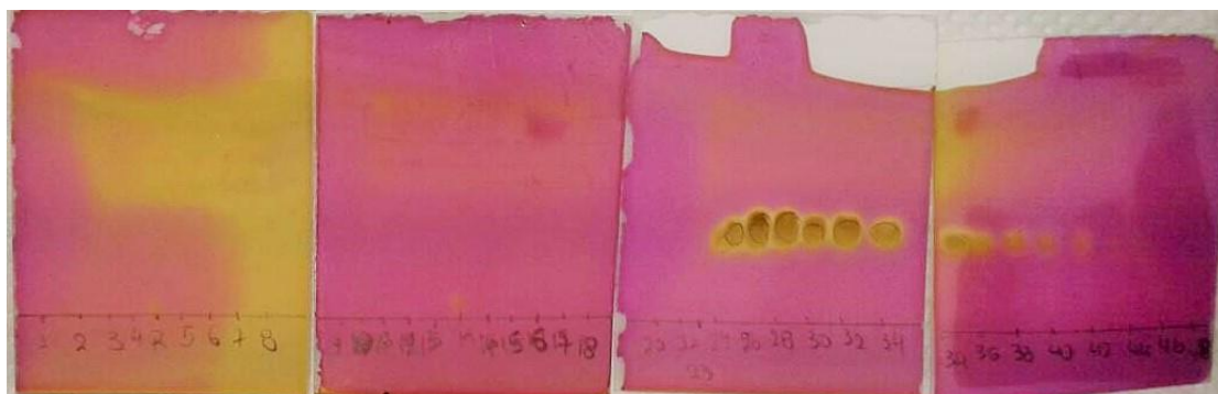
Image 1: TLC plates of the fractions eluted during the chromatographic separation of the reaction mixture revealing that the maleimido-protected initiator 3 was eluted in fractions 23-44 which were combined, placed in a round bottom flask and, upon removal of the solvent under reduced pressure, yielded the final product.
