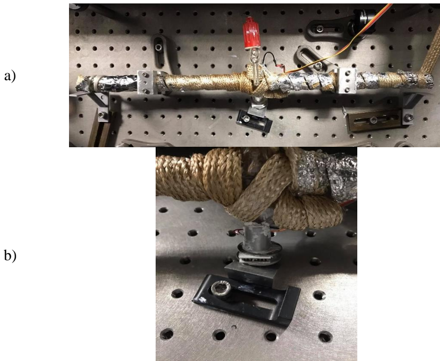
Figure 30: a) Iodine cell wrapped with heat tapes in order to increase the temperature. b) A TEC is placed on the iodine reservoir of the cell and is kept at a specific temperature level below the bulk temperature of the cell. This cold spot then defines the molecular iodine vapor pressure inside the cell.
