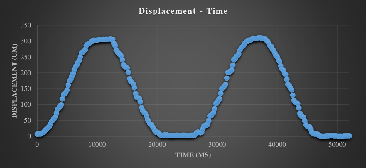
Figure 70: Displacement – Time plot on Shuriken sphere compressed by 75% or 300μm.
