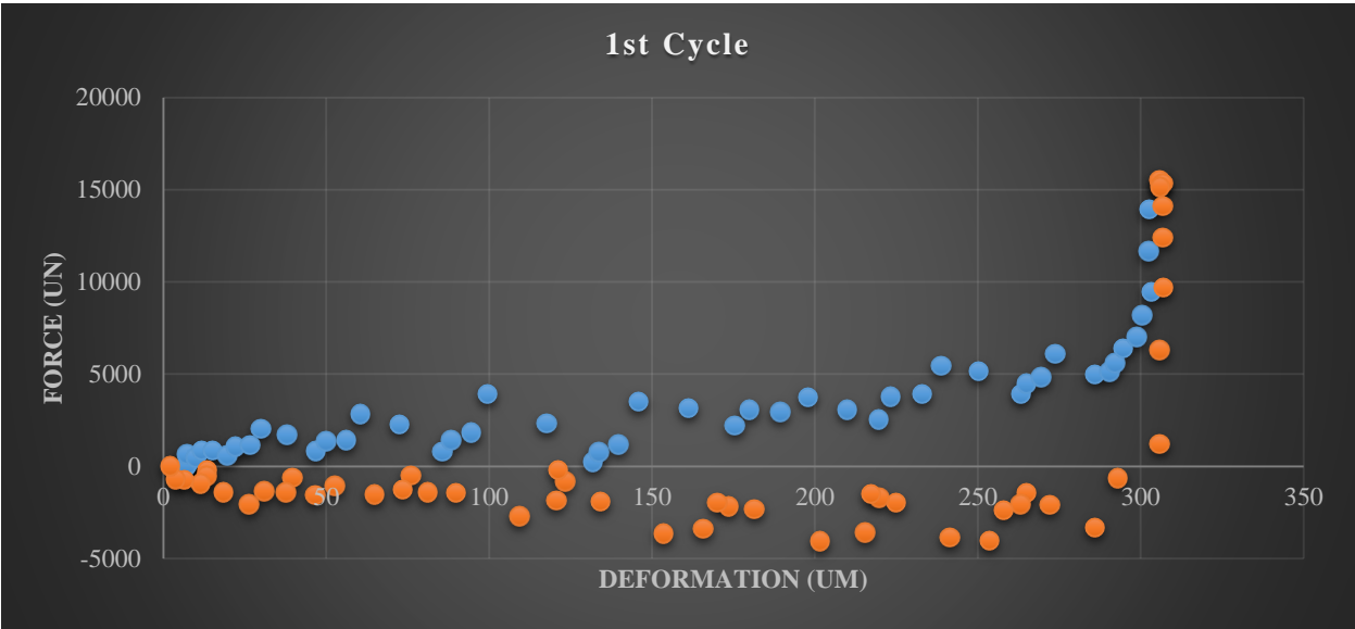
Figure 72: Force – Displacement plot on Shuriken sphere compressed by 75% or 300µm; 1 st cycle, the compression phase was represented in blue, while the recovery phase was indicated in orange on the plot.
