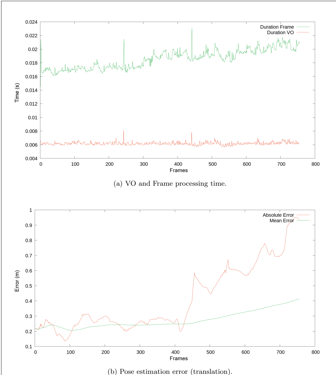
Figure 3.6: Processing Time and translation error from Elastic Fusion in Freiburg1_360 Dataset.
