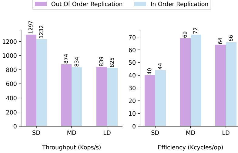
Figure 4.7: Anthus throughput (Kops/s) and CPU efficiency (Kcycles/op) for Load A workload using the SD, MD, and LD KV size distributions.
