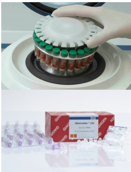
Figure 10. Precellys 2 ml Soft Tissue Homogenizing Ceramic Beads Kit and the homogenizer (Cayman Chemical) (up) and QIAshredder columns (QIAGEN) (down).
