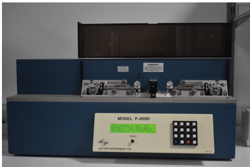
Figure 3.1: Left: Puller for micropipette fabrication. Right: Microforge
