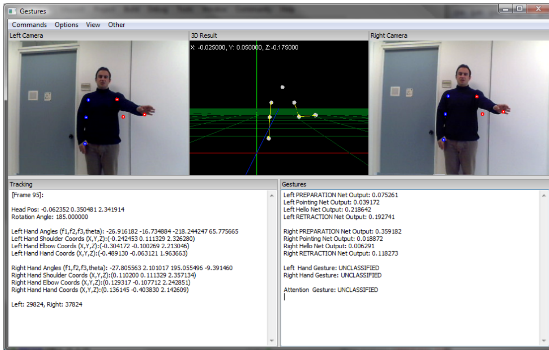
Figure 38: Failure to recognize the performed gesture due to unsuitable resampling deviation.
