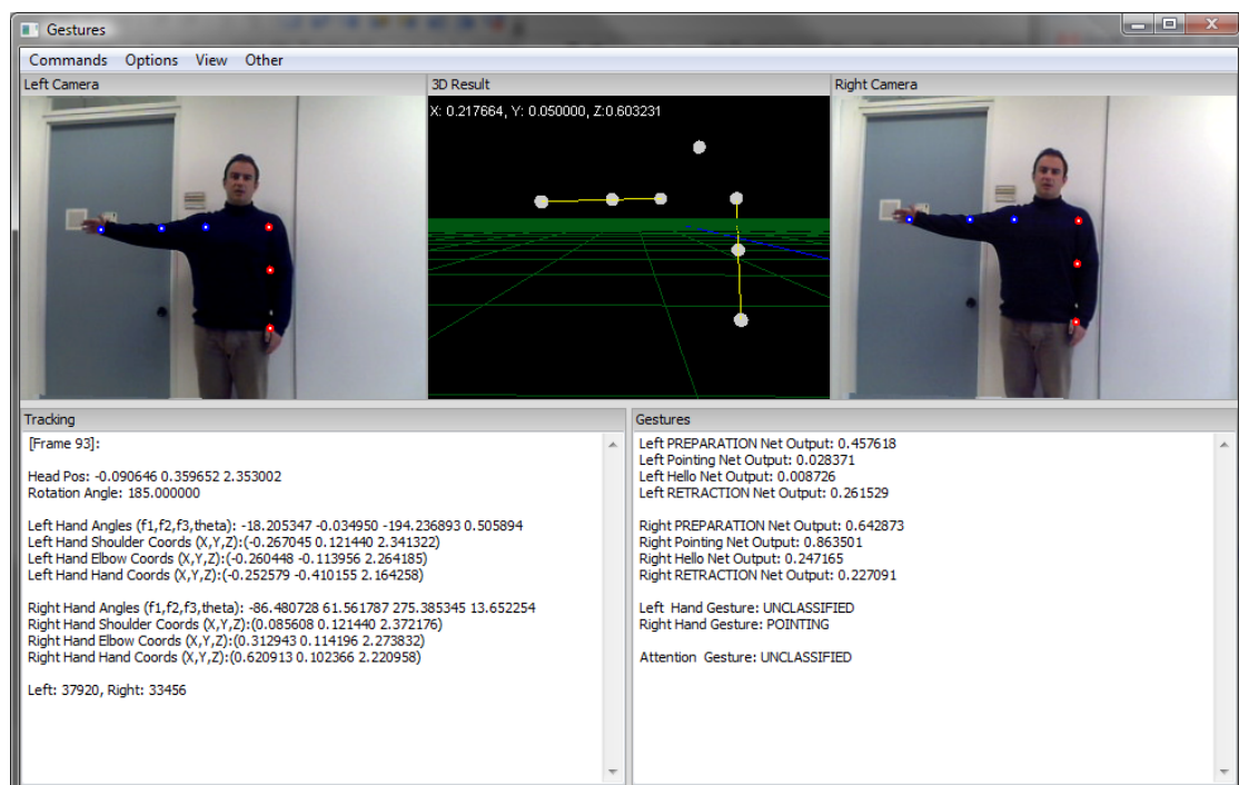
Figure 37: Successful recognition of right pointing gesture.
