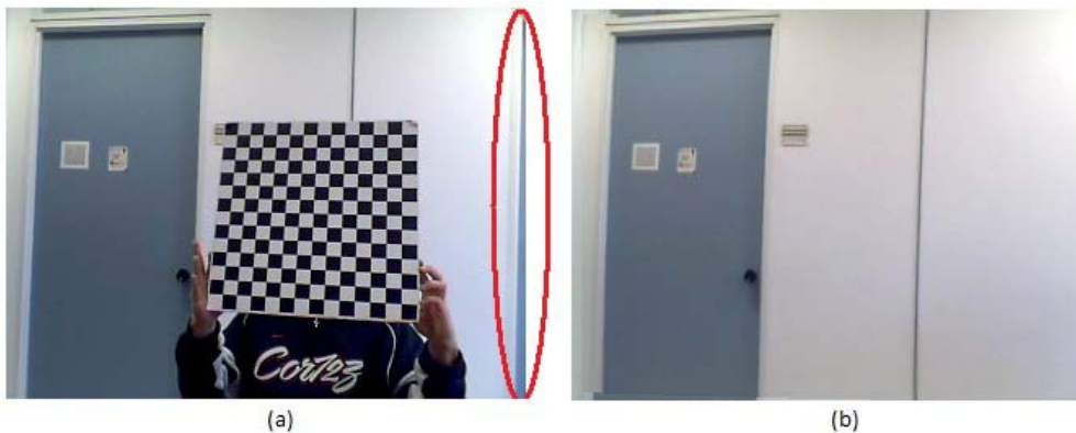
Figure 31: Right Camera moved after calibration.
