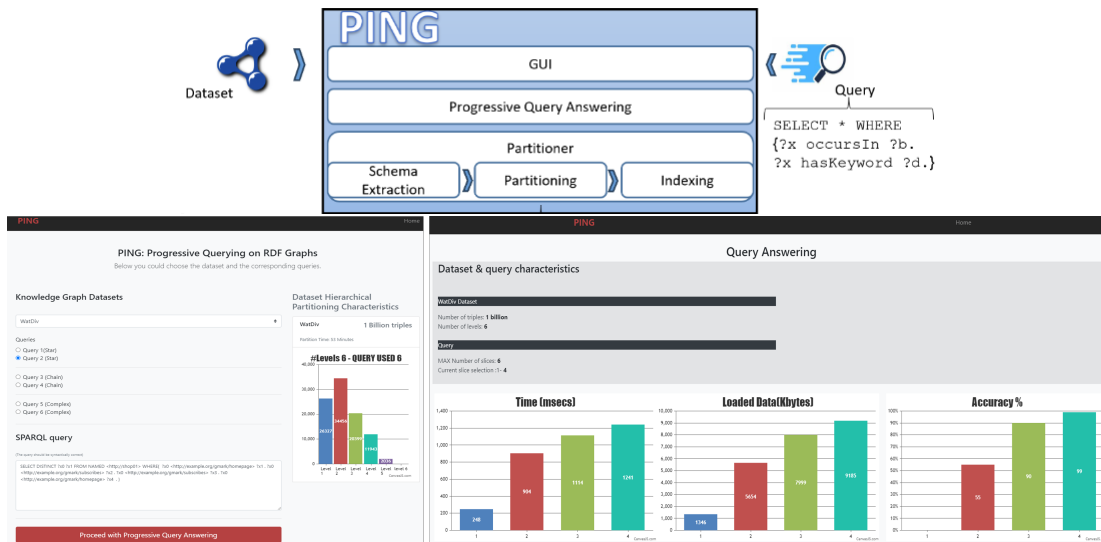
Figure 6.17: System architecture (top), A screenshot of the PING system (bottom).
