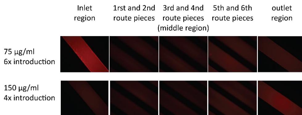
Figure 5.12. Fluorescent images depicting CD45 antibody molecules distribution over the chip surface for the case of design 3 exhibiting increased hydraulic resistance.
