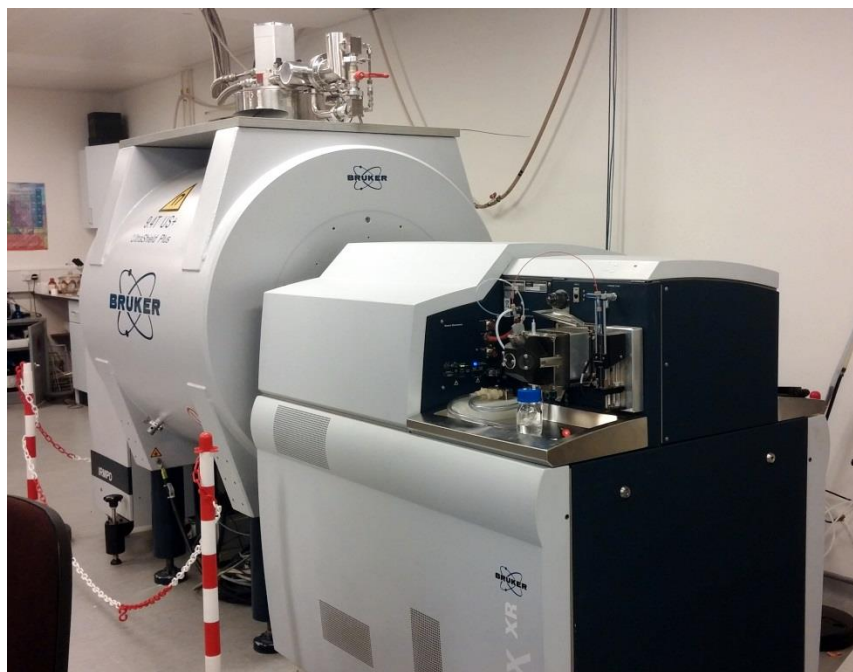
Figure 8: Fourier transform ion cyclotron resonance mass spectrometer (FT-ICR-MS), at university of York
