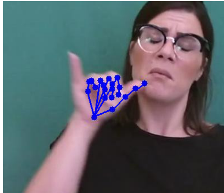
Figure 3.8: Example of an error in 3-D pose estimation. Note that the little finger has not been detected as being extended.
