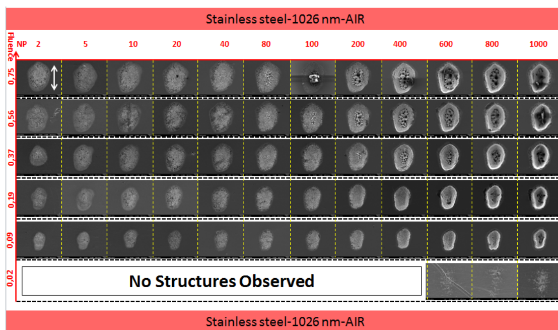
Figure 12: Laser spots on the surface of stainless steel after irradiation with 170fs pulses of 1026 nm. Various self-assembled structures are formed depending on the beam fluence and number of pulses.
