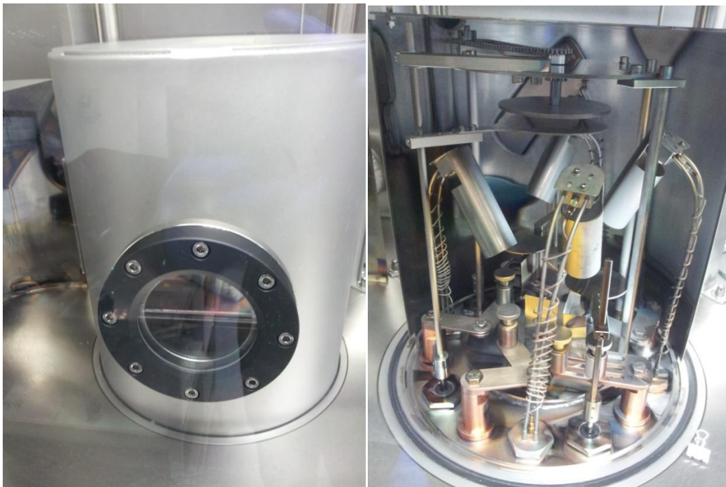
Figure 3-6 The MB-EcoVap evaporator under high vacuum (left) and with the vacuum chamber open (right).
