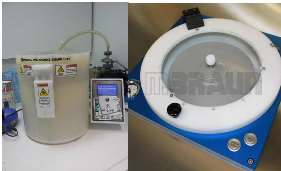
Figure 3-3 The WS-650-23 by Laurell (left) and the MB-SC-200 by MBraun (right) spin coater
