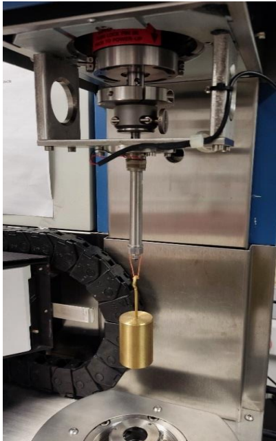
Figure 6.3 Static calibration of the piezoelectric sensor of CPP3+. The photograph shows the fixture with its outer corona and lower cone removed. A standardized weight emulates the normal force. Graph depicts the response for different values of static normal force (weights). The ordinate is the voltage at the charge amplifier output logged by the Picoscope.
