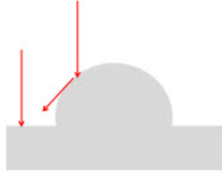
Figure 2.19: Schematic of light reflection off a protrusion leading to enhanced light absorption in the intercone areas
