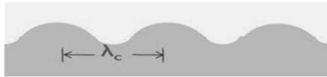
Figure 2.18: Capillary waves excited on a material surface. \lambda_c is the wavelength of the capillary waves. [27]
