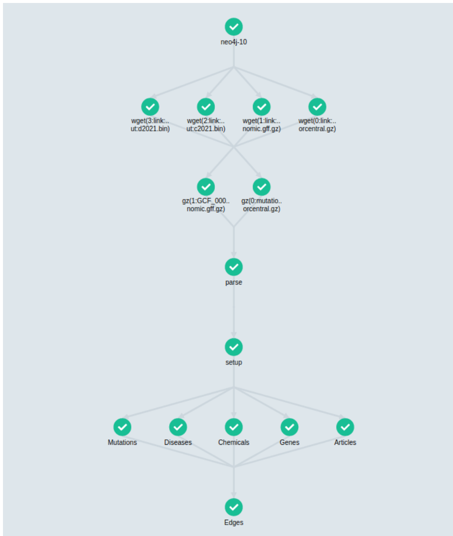
Figure 2.4: “The steps of the building of the graph in Argo workflow”. The first step is the setting up of Neo4j, the second one is the downloading of the required files. The third one is the uncompressing of the files. Fourth step is the parsing of BioCXML files. The fifth one is the preparation of the database for its construction. The last two steps are the importing of nodes in parallel and the importing of edges.
