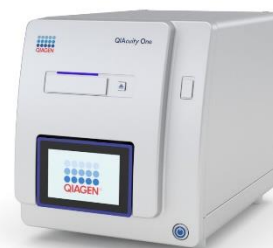
Figure 19: QIAcuity One digital RT-PCR, Qiagen
