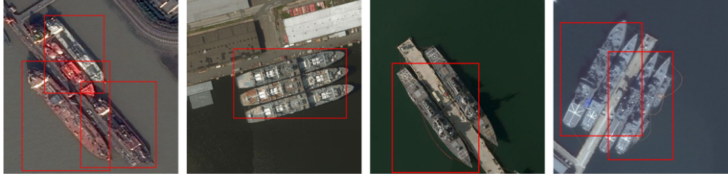
Figure 1.3: Examples of failed detections in remote sensing ship datasets generated from Faster-RCNN with HBBs.
