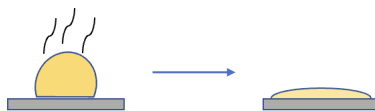
Figure 3.2.1.2: Schematic presentation of the droplet-like sample formation on the substrate, before and after the solvents have been evaporated.
