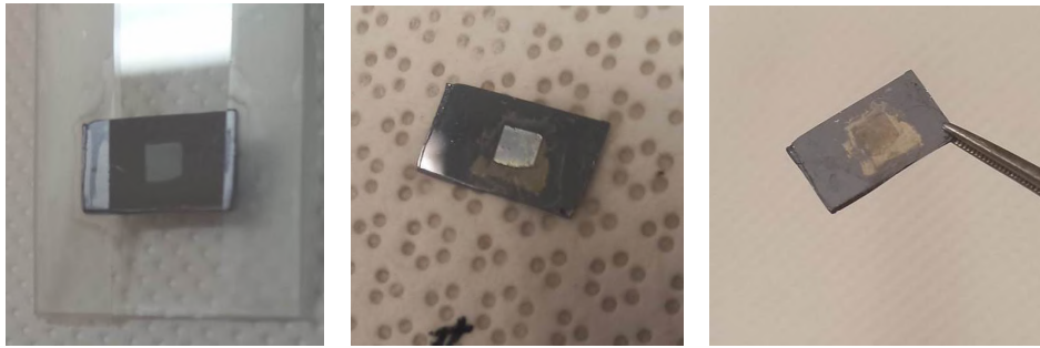
Figure 5.4.1: Images of the final sample, through the metalization process highlighting the change of the surface refractive index and color of the sample.
