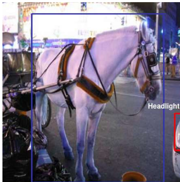
Figure 5.18: Object detector identifies a “Headlight” (red box) with high confidence, but does not relate it to a whole object, triggering an MO error case. The missing object is likely a vehicle (e.g., car), but such object is not annotated in the dataset. Examining such cases may reveal incorrect or missing annotations in the dataset.
