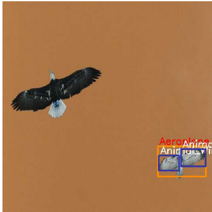
Figure 5.4: Error Case O example. The error is triggered by the whole object “Aeroplane”. This happens because “Aeroplane” is detected with low confidence and is spatially associated with the bounding boxes labeled as “Animal wing”, which have been detected with high confidence.
