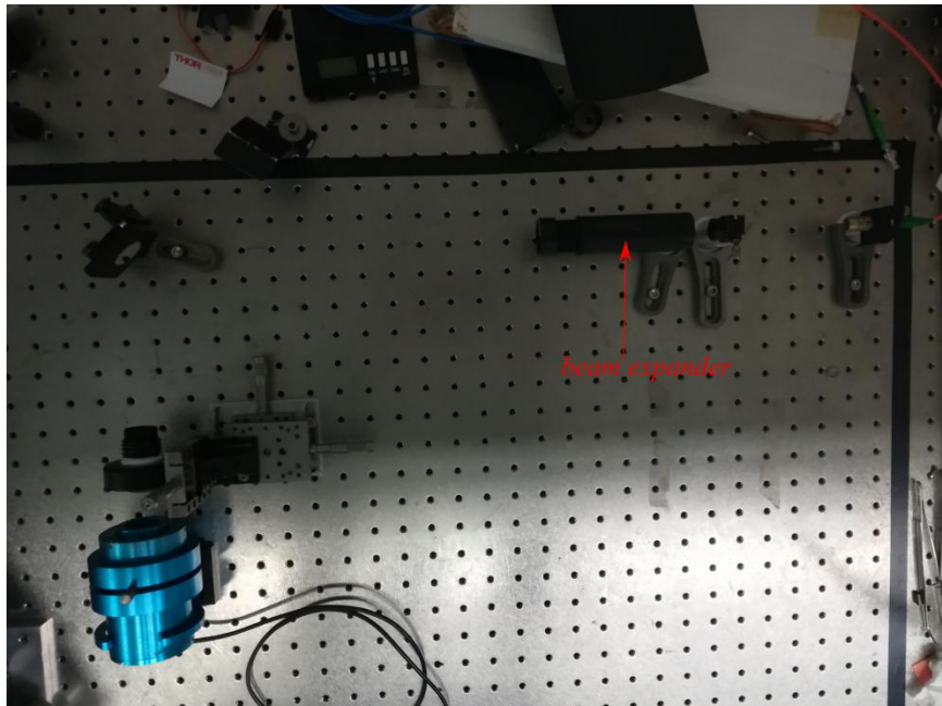
Figure 2.58. Photograph of the total optical setup with the 3x beam expander.
