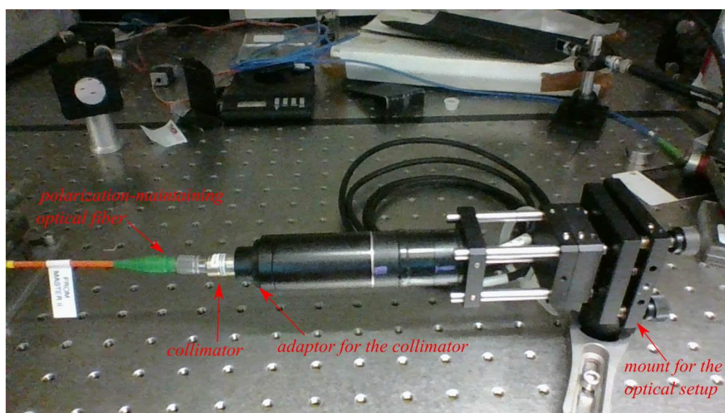
Figure 2.61. A photograph of the test that we made in order to align the Wollaston prism with the photodiodes and check if the optical setup is able to detect the signal.
