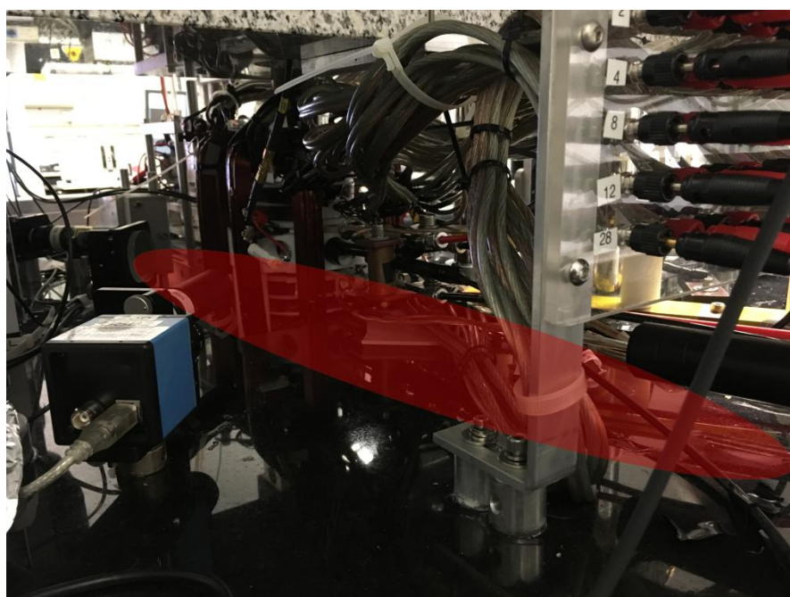
Figure 2.37. An edited photograph that shows the available for new optical elements space. In the optical design process we had to take care about the positions of the other optical elements
