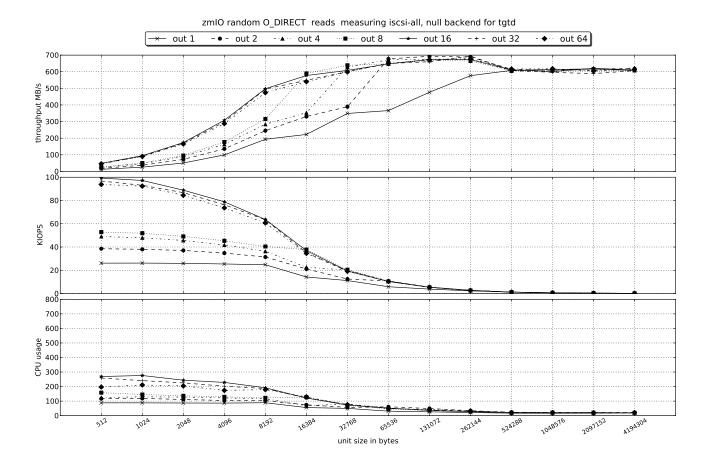
Multiple lines present the varying queue depths for outstanding I/O operations It is notable that performance with only one outstanding operation is low, but scales well while increasing it up to 16 outstanding operations. Performance also increases by increasing the I/O operation unit size (data being transferred per I/O request) up to 256 KB. Nevertheless, *The performance cap for tgtd seems to be around 700 MB/s and 100 K IOPS.*
