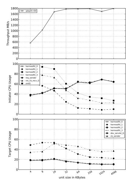
Ramdisk RDMA Read no-memcpy, qdepth=64, Multiedge threads 4 CPU Utilisation Breakdown
