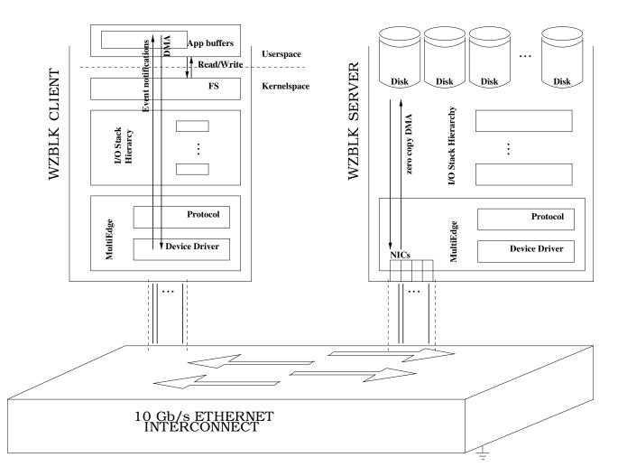
WZBLK, in summary, is a thin glue layer, between Multiedge [4], utilised as the communication protocol and Violin [7] block-layer virtualisation framework, which facilitates the integration of networking support to the exported block device. With primary goal the saturation of today's fastest Ethernet network technology, it boasts simplicity in order to achieve low overhead per operation and scalability in both CPU cores and network links.
