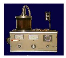
Fig. 41: A sputter coater usually coats the sample with gold atoms. The purpose is to make non-metallic samples electrically conductive.
