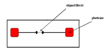
Fig. 47: Preparation of fibroin stalks for X - ray fiber diffraction. Two glass rods are stabilized with plasticine. The fibers are being aligned between the rods
