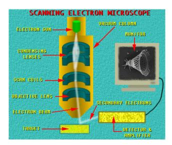
Fig. 40: Image of a typical SEM
