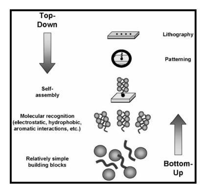
Fig.1: The comparison of Top – down and Bottom – up processes. In the top – down process there is the patterning of assemblies through lithographic techniques; in the bottom – up process there is the formation of well – ordered assemblies through molecular interactions of simple building blocks. [1]
