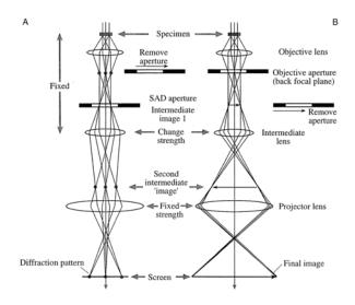
Fig. 42: Imaging to the electron beam in SED comparing to simple imaging [Williams, Carter].
