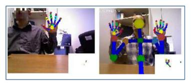
Figure 20 Left: Detection and tracking of only 1 hand and its fingers. Right: Integrated 3D detection and tracking of upper body and 2 hands/fingers.
