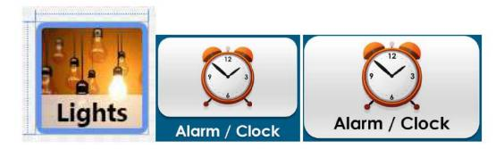
Figure 31: The tile button comprising a background image and a label. Tile buttons can have different appearances, colors and sizes based on the respectively selected styles and can be activated using any of the available modalities as specified into the application's ACTA script.
